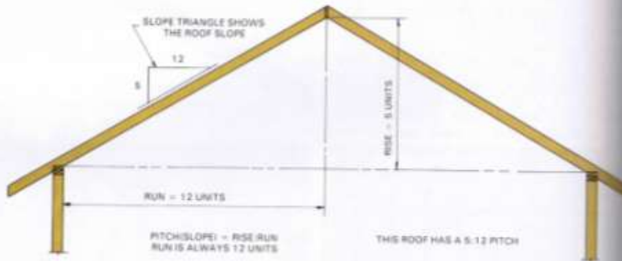
Fig. 17-7. The roof slope diagram represents the relationship of the rise to the run.
